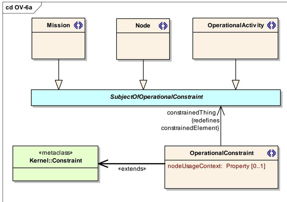
**Figure 3-18: MODAF Meta-Model Excerpt for OV-6a**
