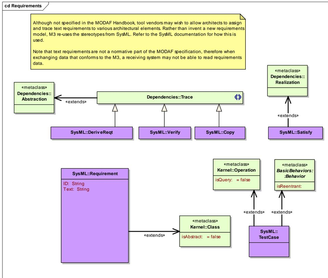
**Figure 3-6: MODAF Meta-Model Excerpt for Requirements**
