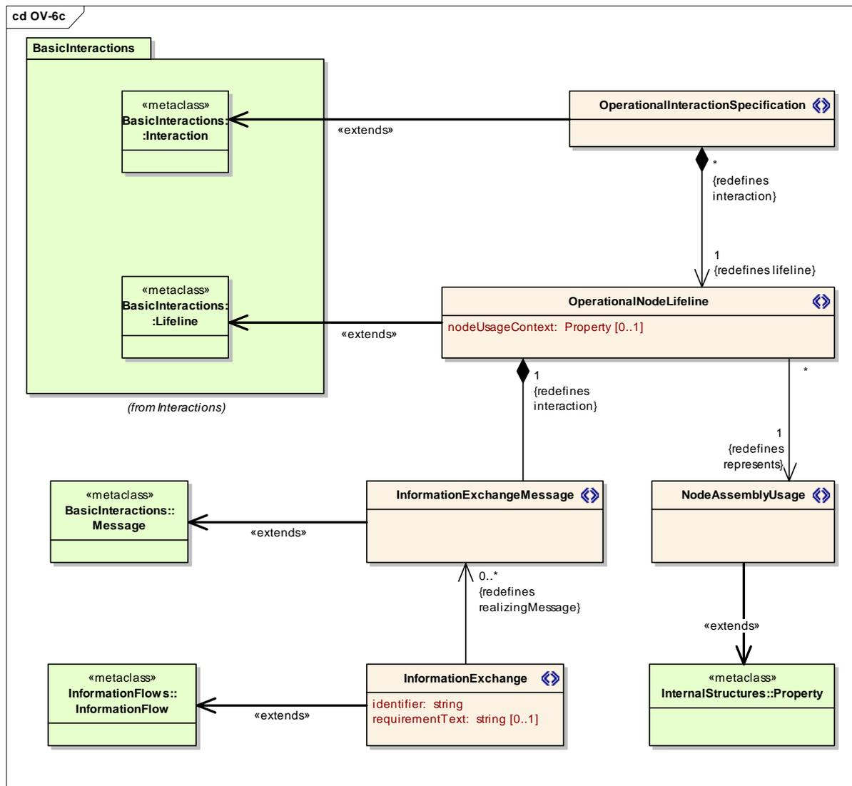
Figure 3-20: MODAF Meta-Model Excerpt for OV-6c
