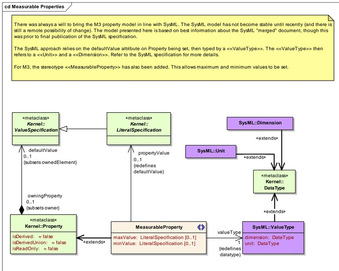
**Figure 3-5: MODAF Meta-Model Excerpt for Measurable Properties**
