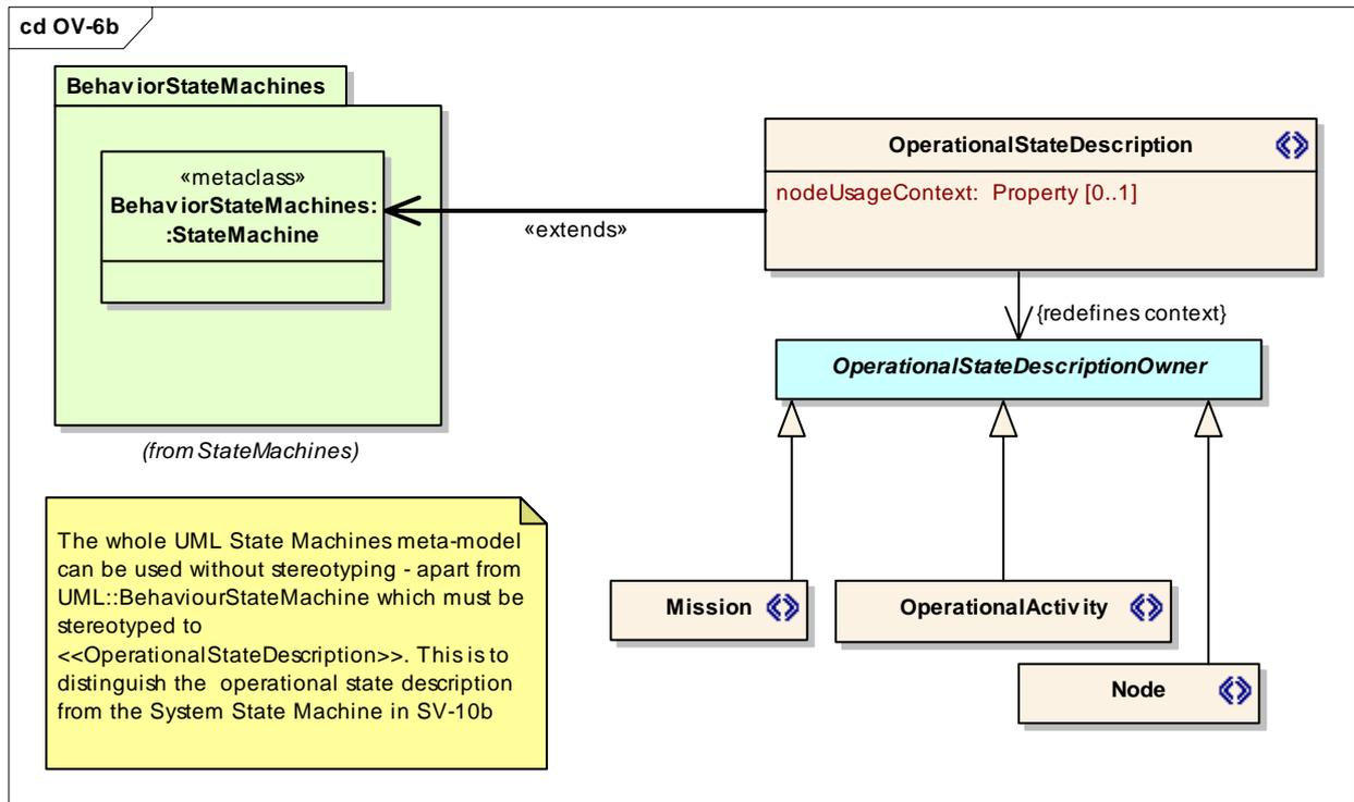
**Figure 3-19: MODAF Meta-Model Excerpt for OV-6b**
